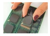
11- Gently place the property conditioned part aligning the balls of leads oh the part with the filled appertures.
