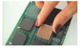
5. Align StencilQuick<sup>TM</sup> by positioning the diagonally opposite corner apertures over the corresponding pads. Note: Ensure thar the pads are centered in the apertures.
