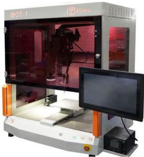
iBot-1 Can handle PCBs up to 430x420mm
