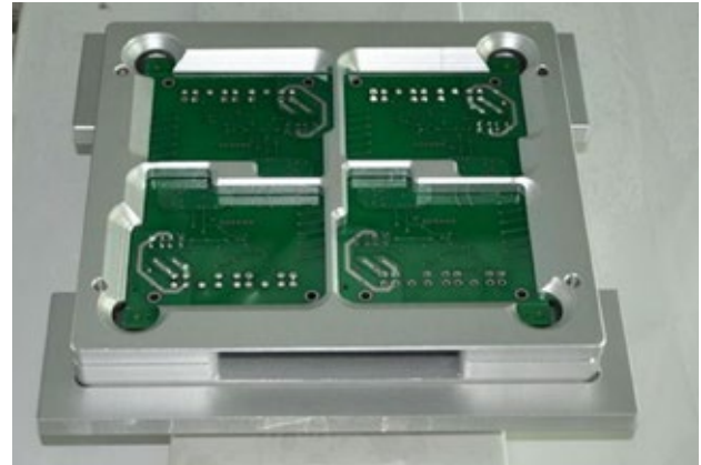
Customerized fixture according to customer's requirement (option).
