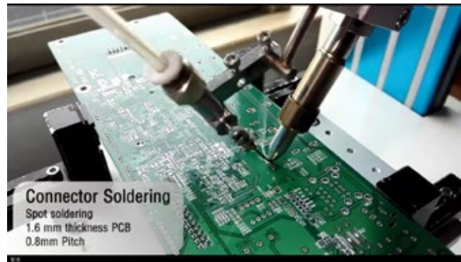
Fine pitch soldering point
